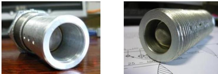
Fig. 2 Two versions of special holder for CO probe [13]
